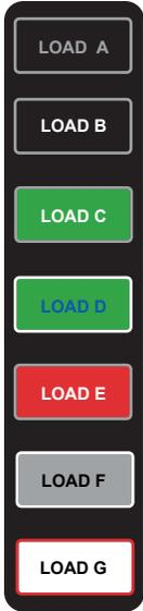
This is a DC Breaker (ECB) which is currently not active. The distribution panel is most likely not receiving any DC power.
