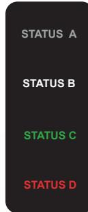
This is a system status indication that is currently inactive. System status indication signals come from a System Monitor (SIU). The SIU is most likely not receiving power or not connected to the network.
